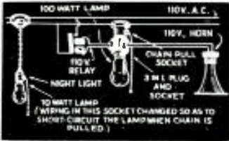
Fig. 1. A novel burglar alarm made from a "dimmer."
