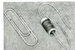
Above, resistor broken to show construction. Below, size comparison. (859)
