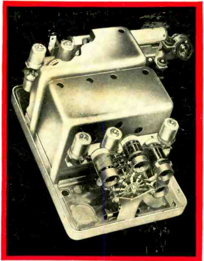
A cut-away view of the underside of SENTRY BOX showing coil mountings and PERMALINERS. Note the clean wiring and short, rigid leads.
